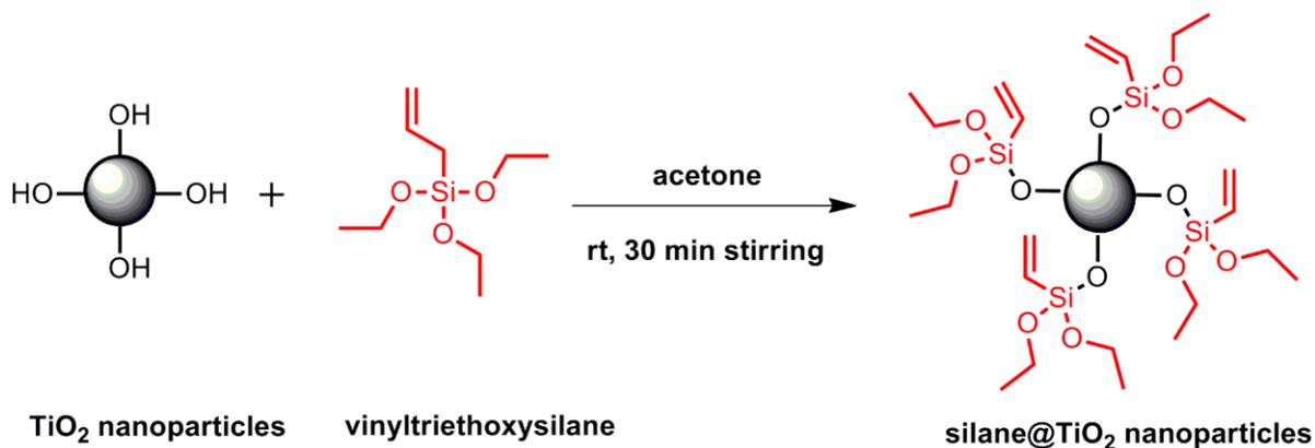
**Scheme 1.** Schematic route for the synthesis of the silane@TiO<sub>2</sub> nanoparticles.
