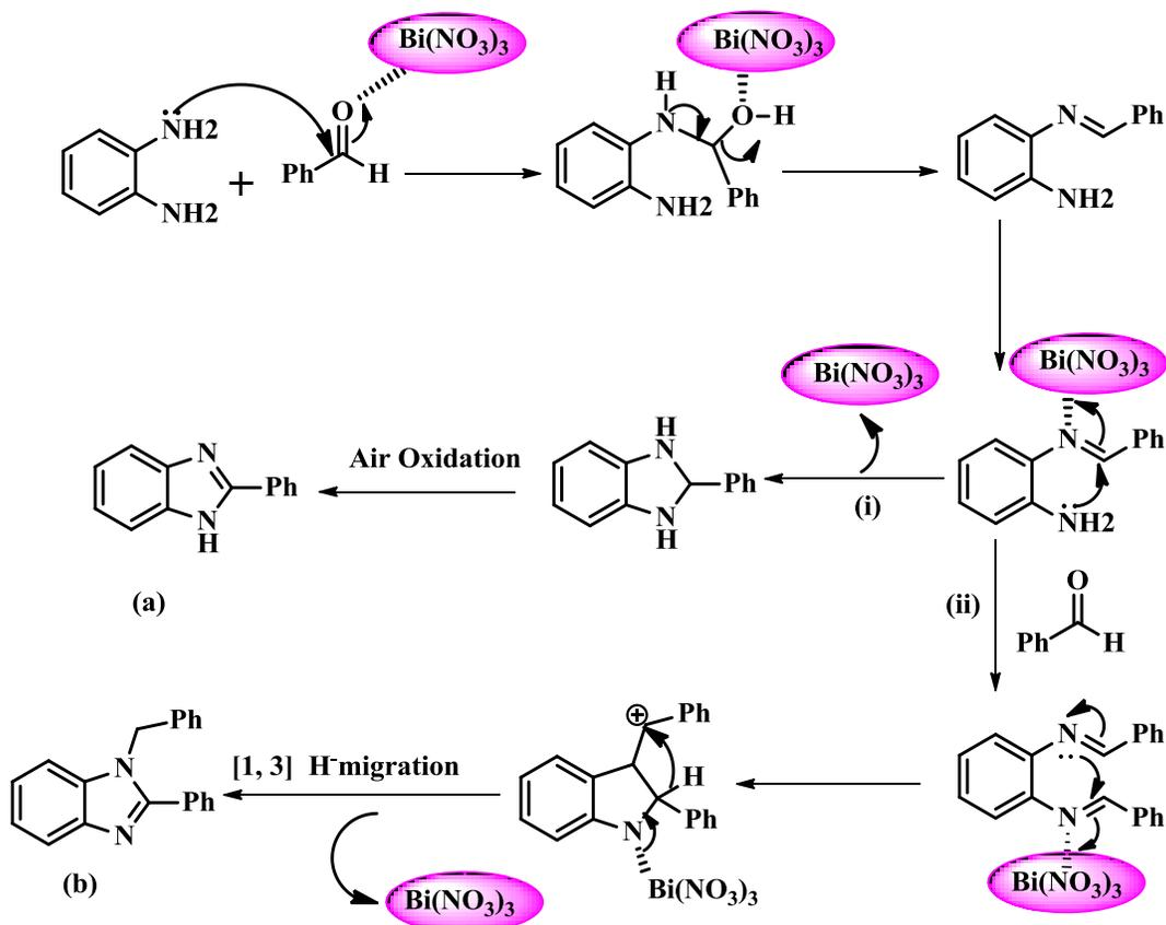
**Scheme 3.** Plausible mechanism for synthesis of (i) 2-substituted benzimidazoles (a) and (ii) 1,2-disubstituted benzimidazoles (b).
