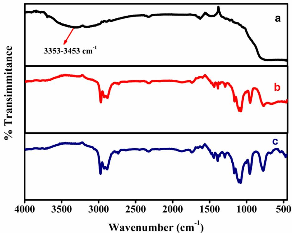
**Figure 1.** FT-IR spectrum of (a) TiO<sub>2</sub>, (b) silane@TiO<sub>2</sub>, (c) vinyltriethoxysilane.
