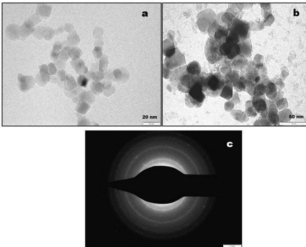
**Figure 5.** (a, b) TEM images  $\text{TiO}_2$  and silane@ $\text{TiO}_2$  nanoparticles. (c) Selected area electron diffraction pattern of silane@ $\text{TiO}_2$  nanoparticles.
