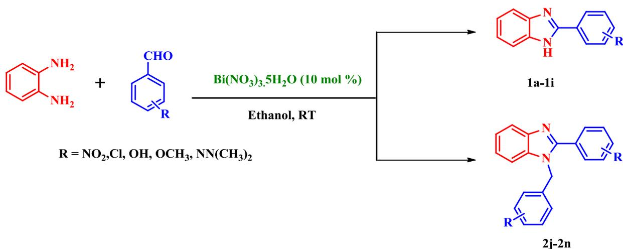
**Scheme 1.** Bismuth nitrate mediated synthesis of 2-substituted benzimidazole derivatives.
