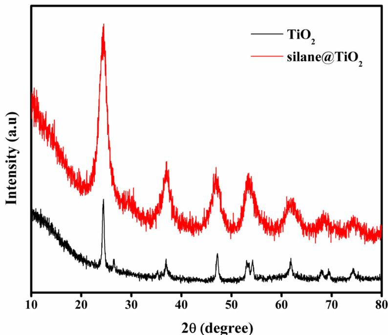
**Figure 2.** XRD pattern of  $\text{TiO}_2$  and  $\text{silane@TiO}_2$  nanoparticles.
