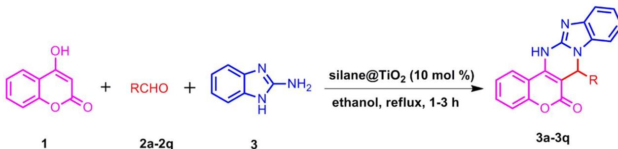
**Scheme 2.** Synthesis of benzo[4,5]imidazo[1,2-a]chromeno[4,3-d]pyrimidin-6-one using silane@TiO<sub>2</sub> nanoparticles.
