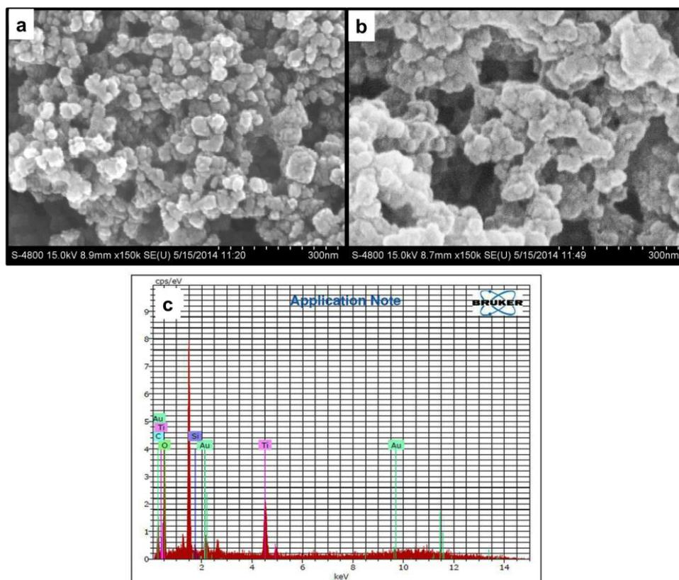
**Figure 3.** (a, b) FE-SEM images of TiO<sub>2</sub> and silane@TiO<sub>2</sub> nanoparticles, (c) EDX spectrum of silane@TiO<sub>2</sub> nanoparticles.
