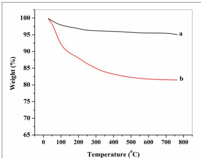
**Figure 4.** TGA thermograms of (a) TiO<sub>2</sub> and (b) silane@TiO<sub>2</sub> nanoparticles under nitrogen atmosphere at a heating rate of 10 °C/min.
